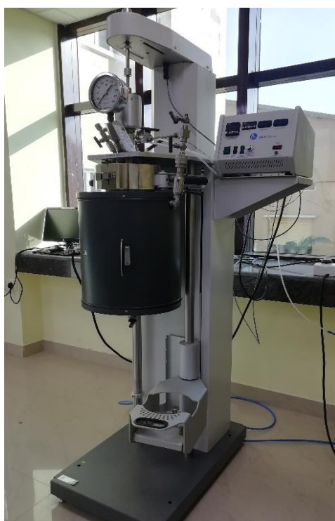
Figure 9. Parr pressure reactor 7.5 liter capacity
